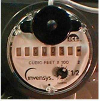
This is a Itron (Sprague/Schlumberger/Actaris) Metris 250 gas meter with an encoded index. The index reads 3 x100 or 300 Cubic feet. The VL-9 would simply read 3, so you would need to add two zeros or put a sticker on the unit that says "x100 CuFt".
