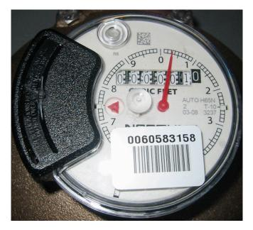
This is a Neptune 2" T-10 Register that reads in CuFt x 10 or 10 CuFt. Since the reading on this register is 10 Cuft, it would be rounded down to 0. If for example it read 34790 CuFt the VL-9 would read 3475 and you would need to add a zero to the reading for the multiplier.
